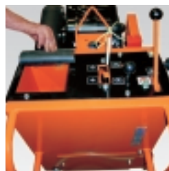
Control panel and the easy access for water supply.
